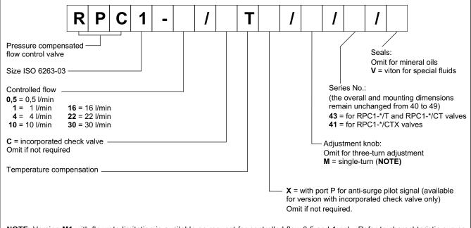
**NOTE**: Version **M1** with flowrate limitation is available on request for controlled flow 0.5 and 1 only. Refer to charachteristic curves diagrams for flow limits.
