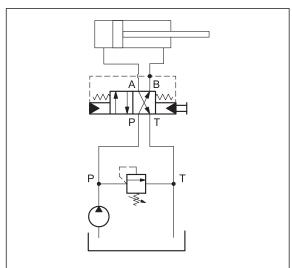
To set the system relief valve correctly, the self-reversing function must be inactive.
