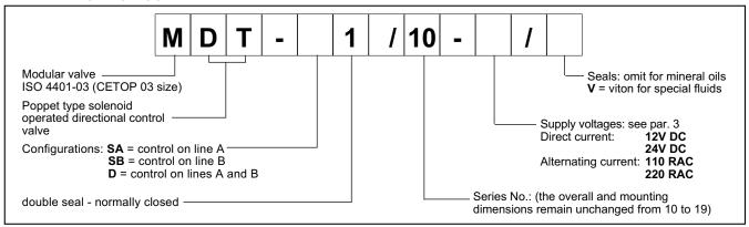
NOTE: The solenoid valves are never supplied with connector. Connectors must be ordered separately. To identificate the connector type to be ordered, please see catalogue 49 000.
