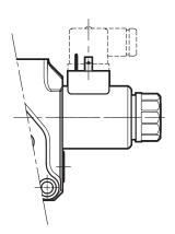
connection for DEUTSCH DT04-2P connector type code  $\mathbf{K7}$
