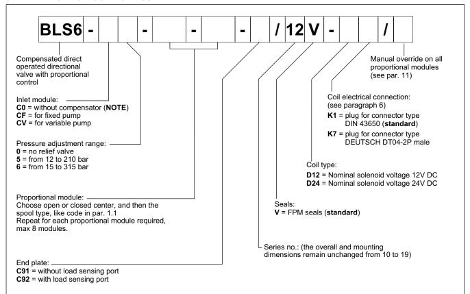
NOTE: The version C0 is available only without the pressure relief valve, with code BLS6-C00/12V.
