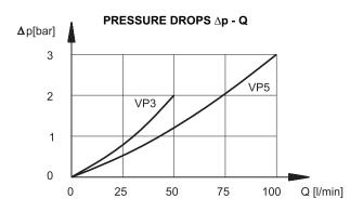
**NOTE:** The curves shown in the graph refer to B→A and A→B flow with the valve released hydraulically.
