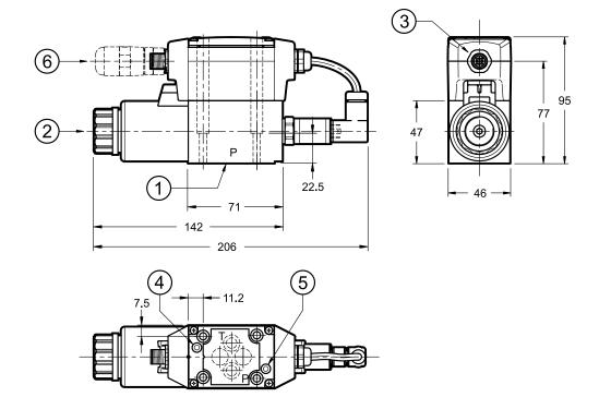
**NOTE**: at the first start up, or after a long period of no use, it is necessary to vent the air through the breather (2) placed at the end of the solenoid tube.
