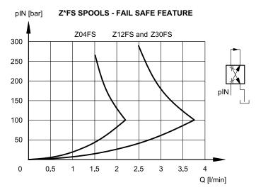
Flow P $\to$ B / A $\to$ T with valve in fail safe position, depending on the inlet pressure.
