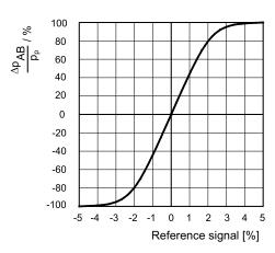
The diagram shows the valve pressure gain, expressed as % of the ratio between the port pressure variation in A or B ( $\Delta p$  AB) and the P system pressure, according to the reference signal.
