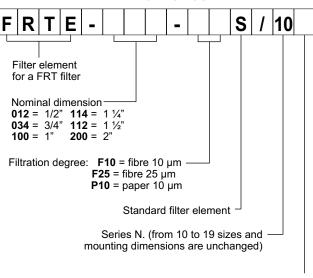
N = NBR seals for mineral oils (standard)V = FPM seals for special fluids (upon request)
