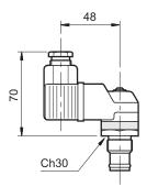
This indicator, apart from giving a visual indication, for example the VPM model, operates by switching an electric contact when the filter element has reached the clogging limit.
