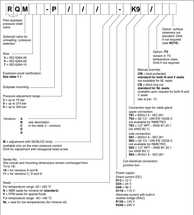
**NOTE**: Valves are supplied with standard surface treatment of phosphating black for the main body and zinc-nickel for the pilot body. The full zinc-nickel surface treatment is available upon request. It is suitable to ensure a salt spray resistance up to 600 h (test operated according to UNI EN ISO 9227 standards and test evaluation operated according to UNI EN ISO 10289 standards).
