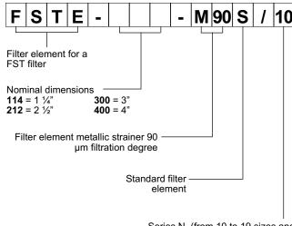
Series N. (from 10 to 19 sizes and mounting dimensions remain unchanged)
