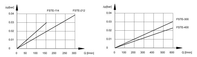
NOTE 2: the filter size has to be selected so that with the nominal flow rate the pressure drop is lower than 0,02 bar.
